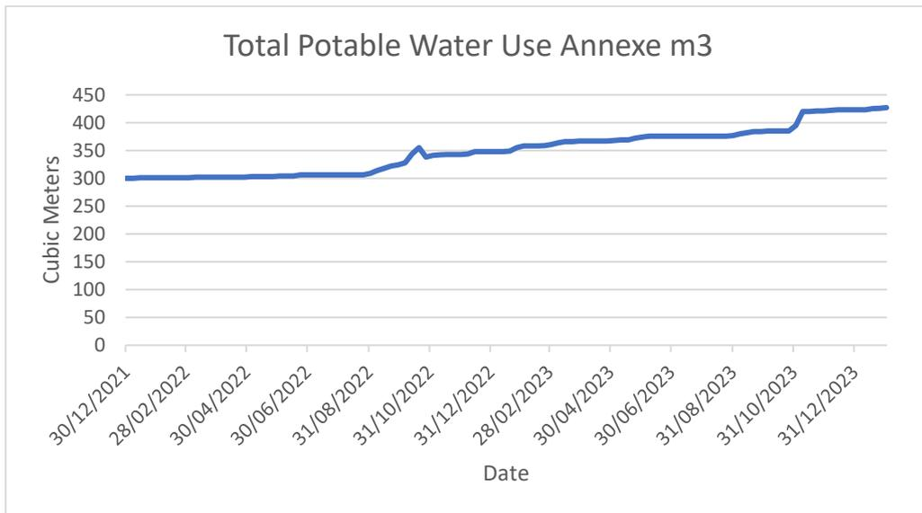
7.7 The low water usage in the annex is due to all toilet flushing coming from the rainwater harvesting system.
